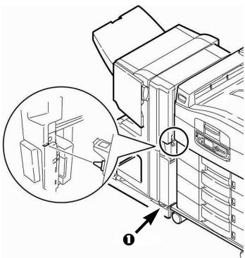
**Note:** If you need to, turn the levellers (①) on either side of the finisher to raise or lower it so the holes and prongs align properly. Make sure the finisher is level.
